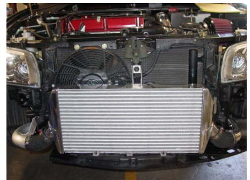
This large heavy 23" x 11 1/2" x 3" intercooler will fit the stock piping and elbows or Injens intake system. Intercooler cores are made in Australia. This intercooler will support up to 750 h/p
