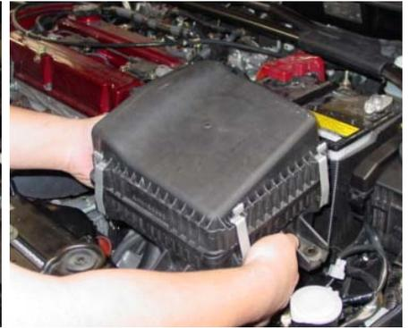
The stock air intake box is removed and the mass air flow sensor is disconnected from the intake box to be used later in the instruction.
