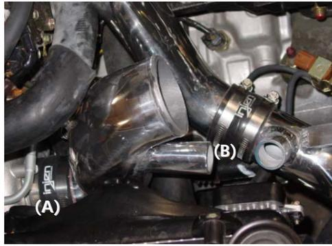
The cast intake (A) and secondary pipe to the intercooler (B) has been installed and ready for the next step.
