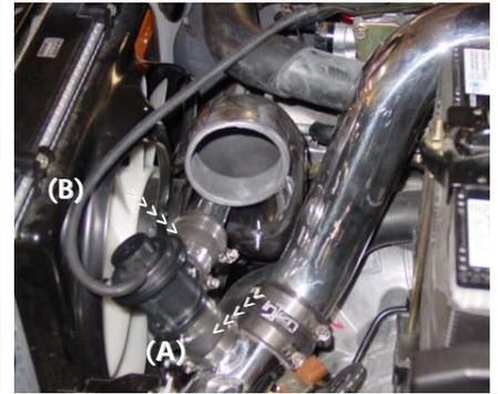
Insert the assembled blow-off valve over the large port on the intercooler pipe(B). Press the other end over the large port on the intake(B). **If another manufacturer's intake is being used some modification will be required.**
