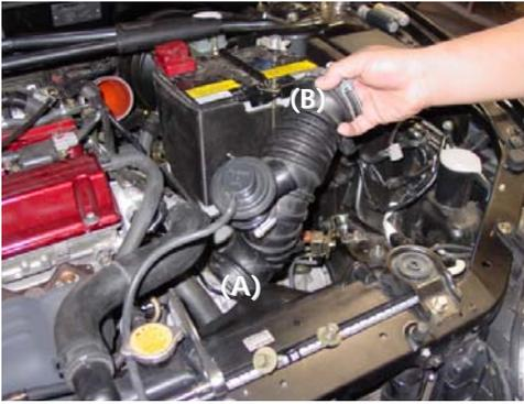
Remove the stock air intake duct connected to the turbo outlet (A) and the air intake box (B). This system must be used with an up graded intake system. **This system cannot be used with the stock air intake system.**
